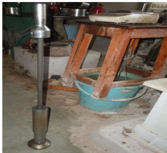
Fig 4.5: Hammer used for compaction
