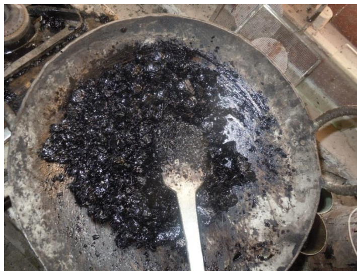
Fig 4.3: Mixing of aggregates, bitumen, zeolite and filler
