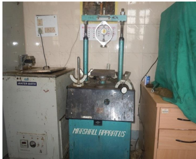
Fig 4.9: Marshall test apparatus
