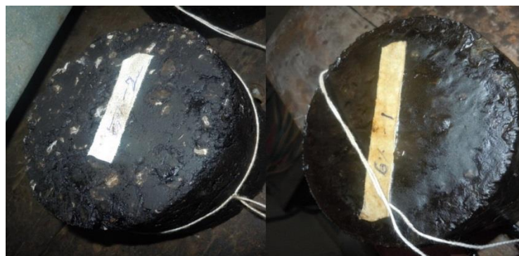
Fig 4.7: Samples before and after wax coating
