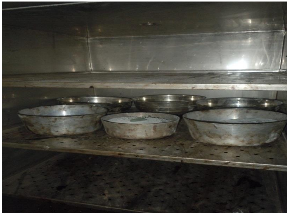
Fig 4.1: Heating of aggregates and filler mixture in oven
