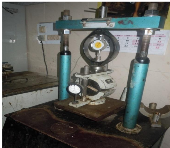
Fig 4.10: Marshall test being conducted with the Marshall apparatus
