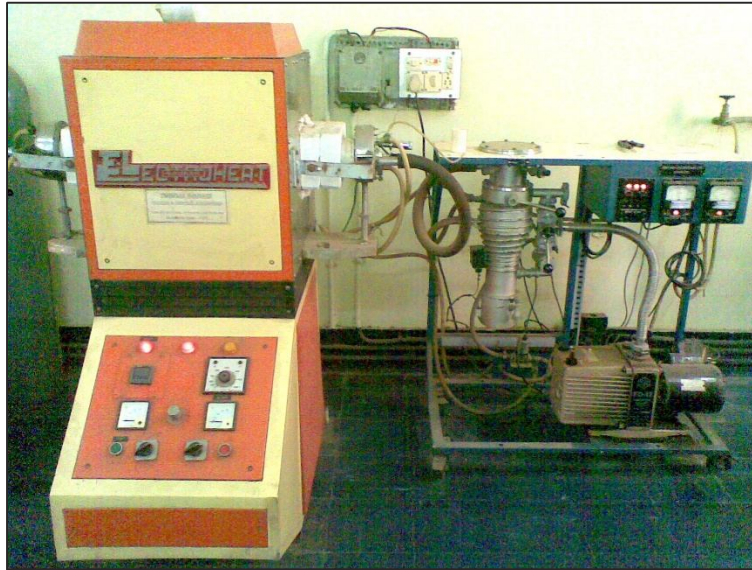
Figure 3 - 3: Experimental Set up for Sintering
