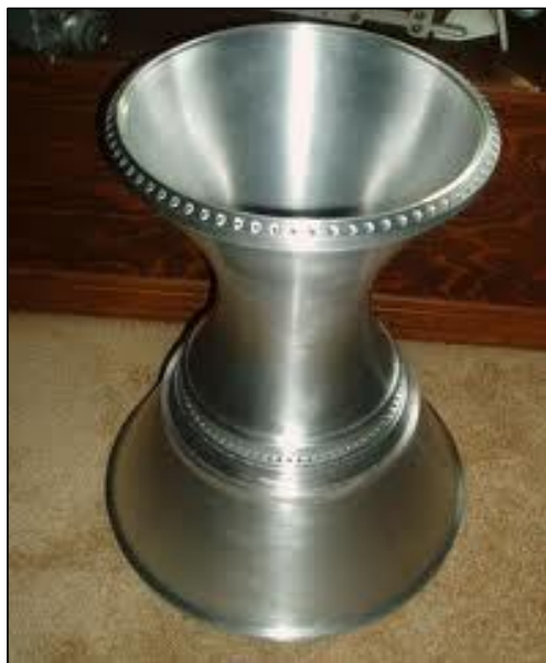
Figure 1 - 3: Shows the thrust chamber lines of the rocket engine components
