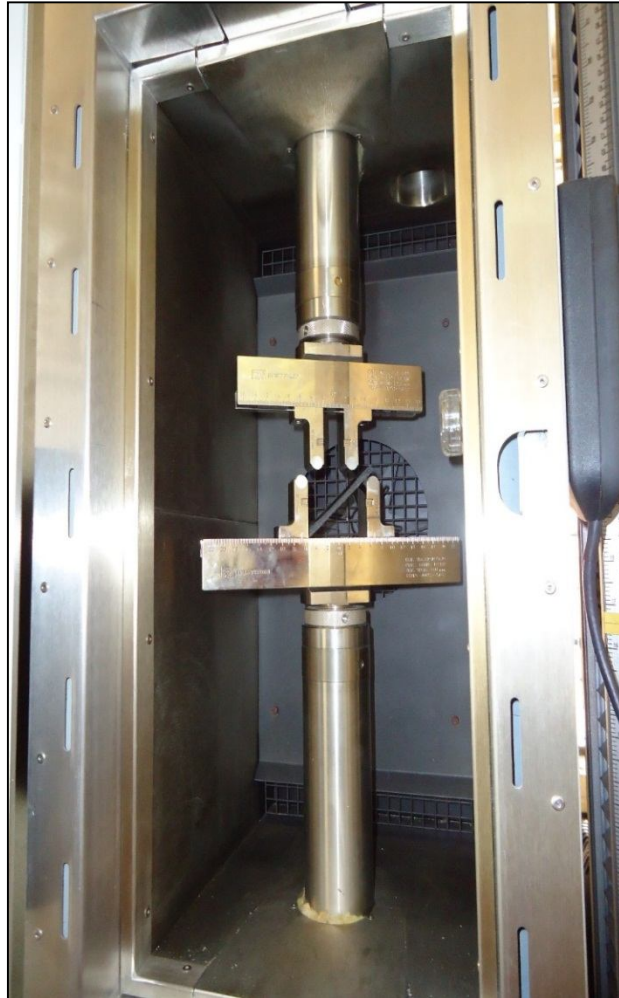
Figure 3 - 5: Shows the set up for 3-point bend test
