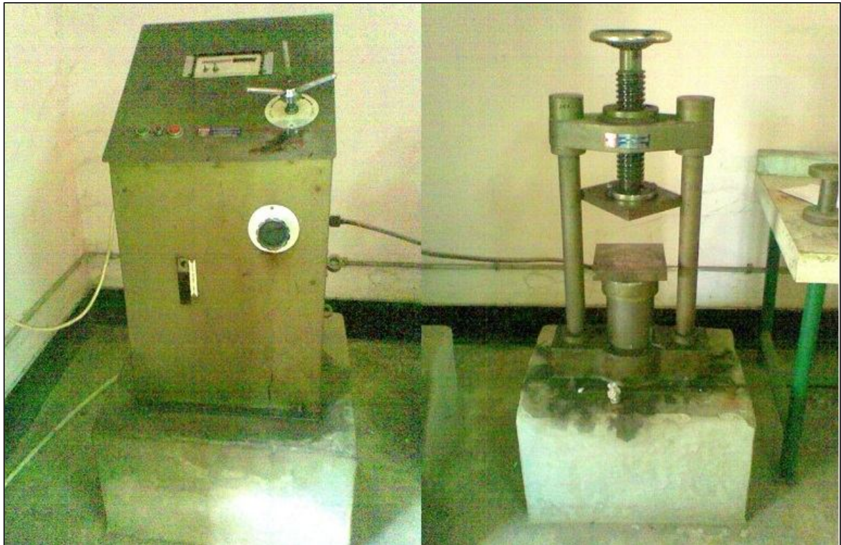
Figure 3 - 2: Experimental Set up for Compaction of sample
