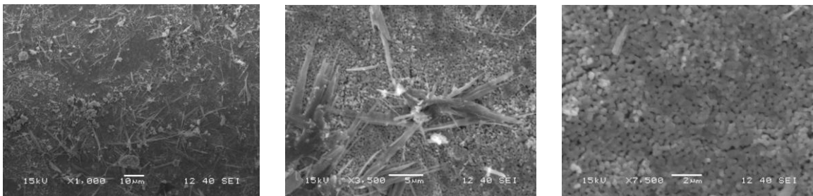
Fig4.4 SEM image of \text{Pr}_{0.75}\text{Na}_{0.25}\text{MnO}_3
