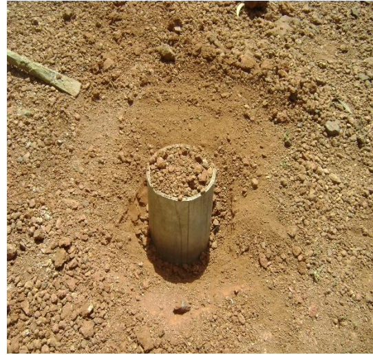
Fig 3.3: Preparation of location of sample collection Fig 3.4: mould with sample
