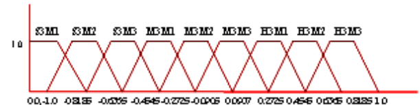
Fig. 5.6(f) Membership functions for relative mode shape difference for first mode of vibration.
