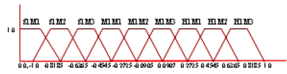
Fig. 5.6(d) Membership functions for relative mode shape difference for first mode of vibration.
