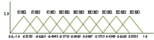
Fig. 5.4(f) Membership functions for relative mode shape difference for first mode of vibration.
