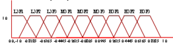
Fig. 5.6(c) Membership functions for relative natural frequency for third mode of vibration.
