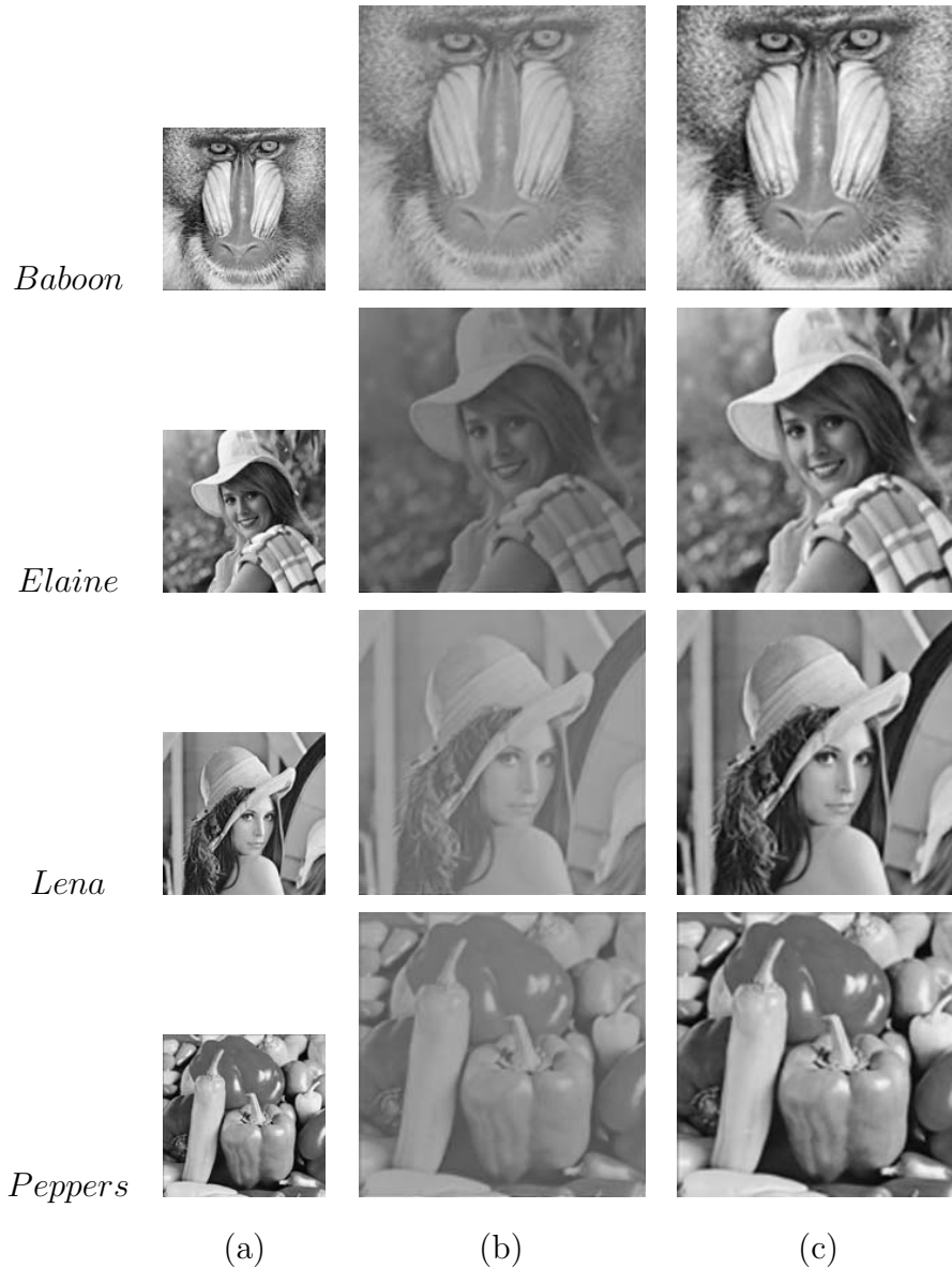
Figure 3.3: (a) input images of resolution 256 \times 256 . (b) DWT SR outputs of resolution 1024 \times 1024 . (c) Proposed method outputs 1024 \times 1024 .
