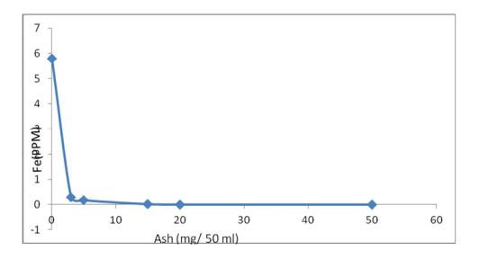
Fig 5.2 Concentration of iron ion versus amount of ash mixture in mg/50 ml of iron solution
