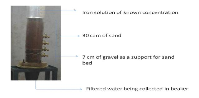
Fig 4.1 Filtration using plane sand as filter media
