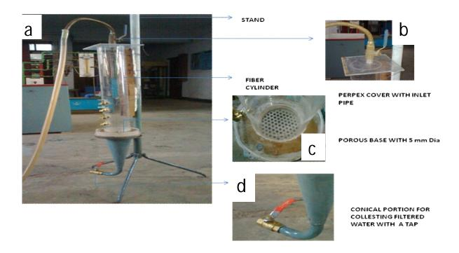
Fig. 3.1(a) Filtration Model, (b) Inlet pipe fitted with the perpex cover, (c) Porous base, (d) Conical portion for water collection
