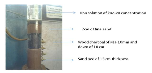
Fig 4.3 Filtration using wood charcoal as adsorption media
