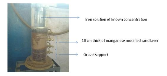
Fig 4.5 Filtration by manganese modified sand
