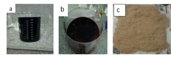
Fig 3.4(a) 0.01N KMnO4, (b) sand soaked in 0.01N KMnO4, (c) oven dry manganese modified sand
