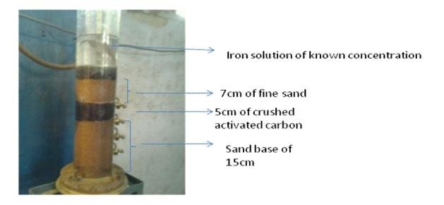
Fig 4.2 Filtration using Activated carbon as adsorption media
