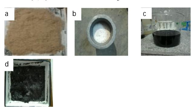
Fig 3.6 (a) Rice husk ash prepared after controlled heating at 500 degrees, (b) RHA soaked with 0.01N HCl, (c) Al(OH)3 coated RHA
