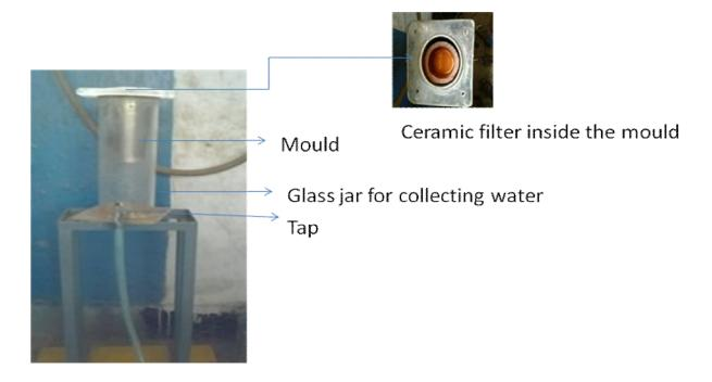
Fig 4.8 filtration of turbid water by ceramic filter
