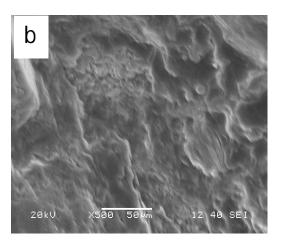
Fig 5.1(a) SEM image of uncoated sand, (b) SEM image of Manganese modified sand with 500 x magnifications
