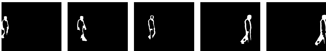
Figure 3.6: Output of frame difference result after noise removal
