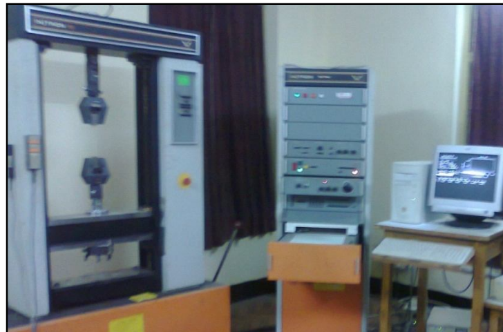
Figure 3.9 Instron Corporation, series IX Automated Materials Testing System 1.26 with specimen
