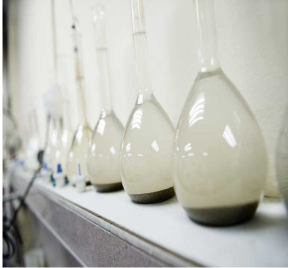
Figure 3.1 Pycnometer with water and pond ash
