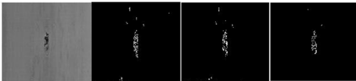
Figure 2.6: (a) Original image, (b) defect detection with \sigma=1 (c) defect detection with \sigma=2 (d) defect detection with \sigma=3
