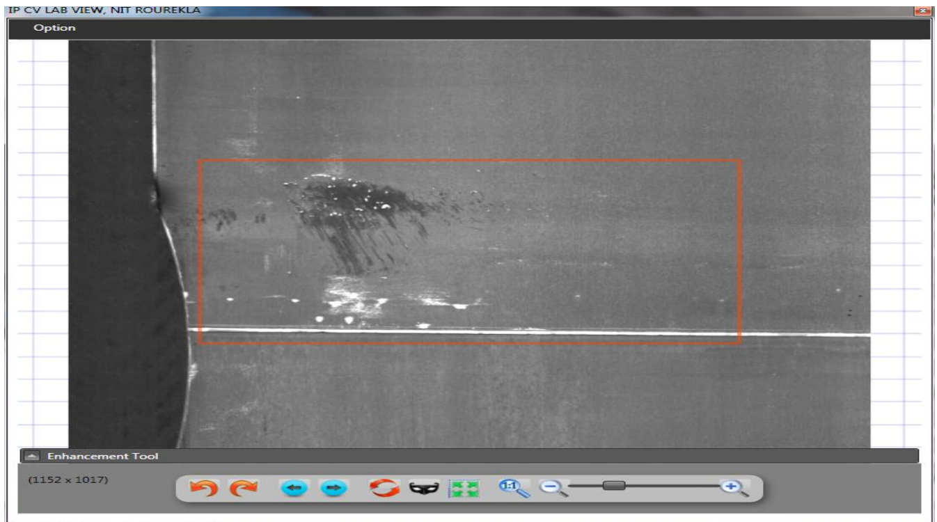
Figure 2.11: Defect detection of weld mark by Proposed method Using visual studio
