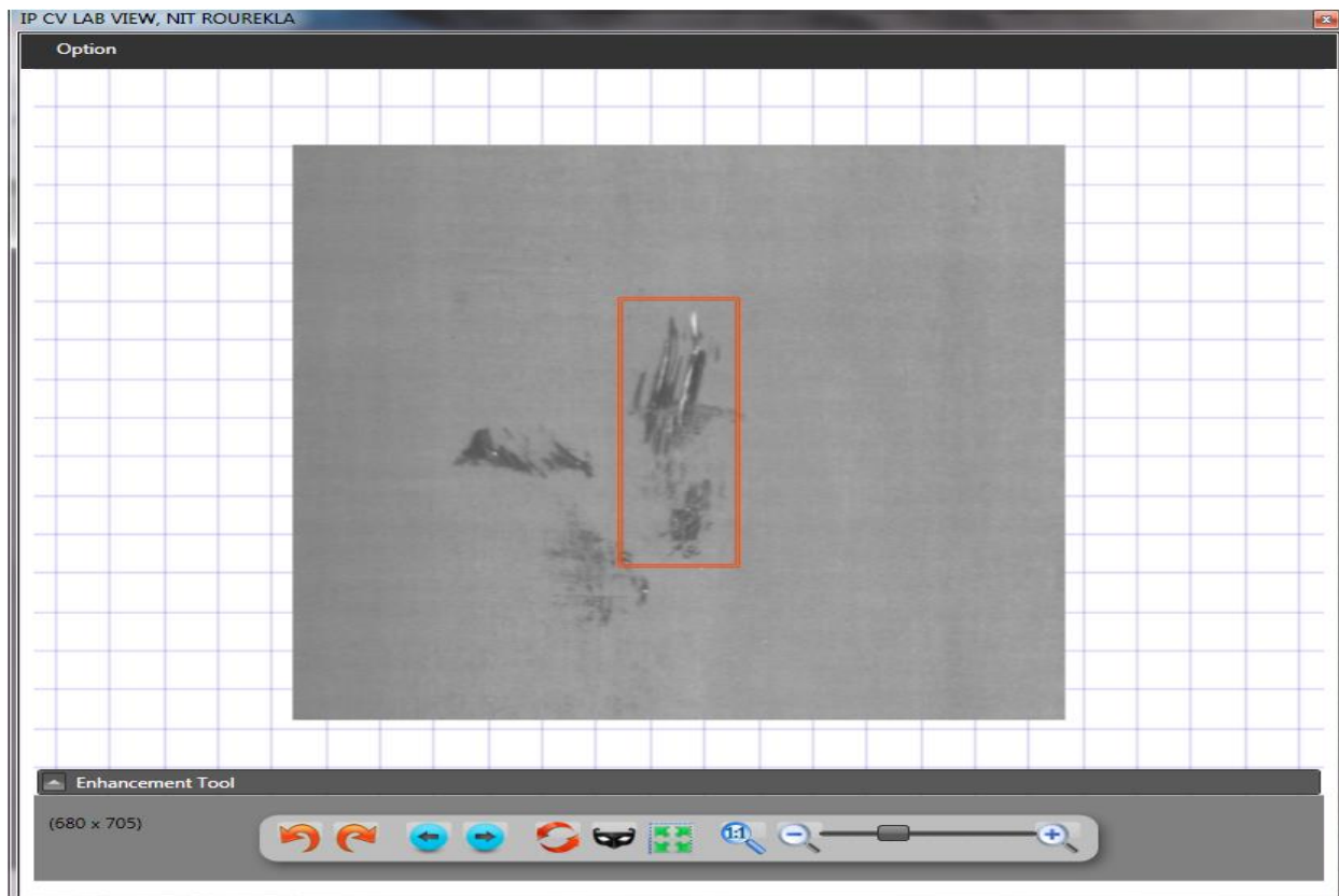
Figure 2.10: Defect detection of roll mark by Proposed method Using visual studio
