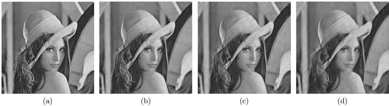
Figure 6.6: (a) Original image, 256 by 256, 8bits/pixel,with MSE = 0 , PSNR = \infty , (b) Restored image of noise var. 0.04, (c) Restored image of noise var. 0.06, (d) Restored image of noise var. 0.08
