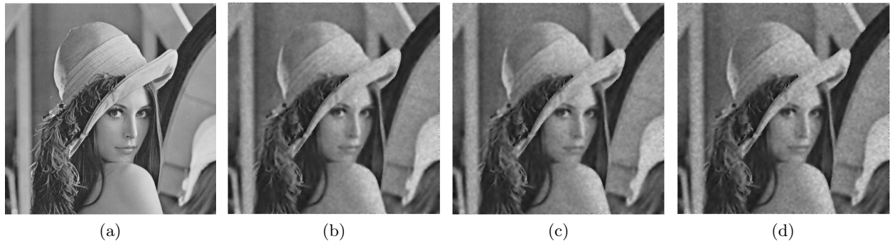
Figure 6.3: (a) Original image, 512 by 512, 8bits/pixel,with MSE = 0 , PSNR = \infty , (b) Restored image of noise var. 0.04, (c) Restored image of noise var. 0.06, (d) Restored image of noise var. 0.08
