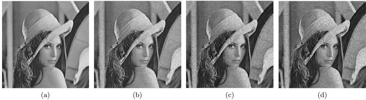
Figure 6.1: (a) Original image, 512 by 512, 8bits/pixel,with MSE = 0 , PSNR = \infty , (b) Speckle noisy image with var. 0.04, (c) Speckle noisy image with var. 0.06, (d) Speckle noisy image with var. 0.08
