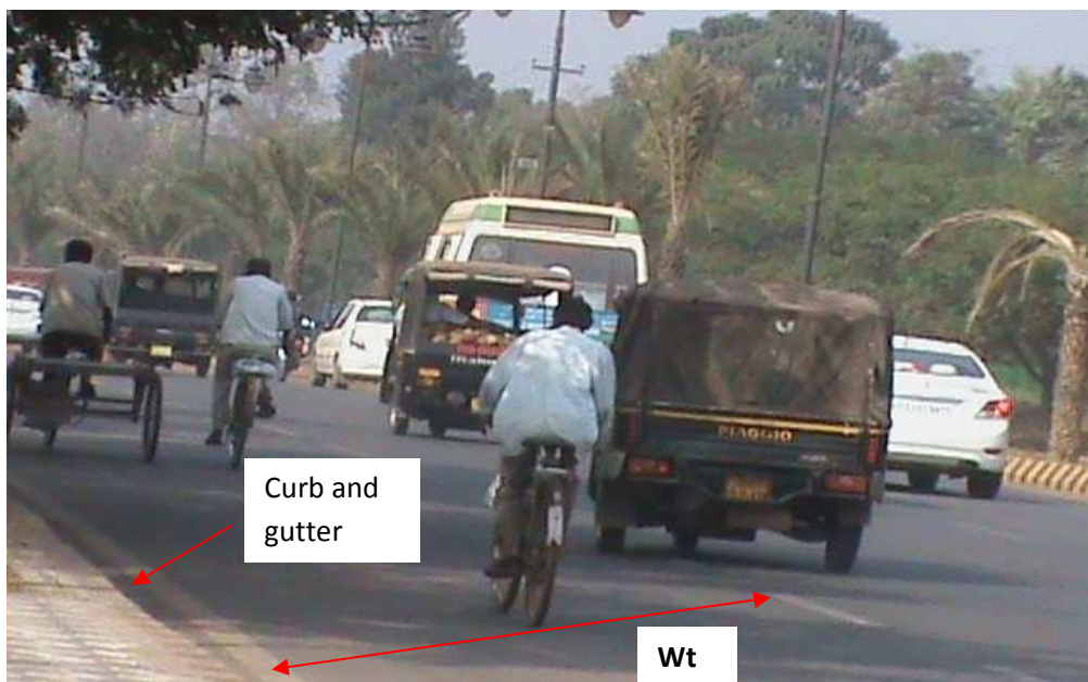
Figure 5.3 Width of pavement for the outside lane and shoulder ( W_t ) (For multilane road)
