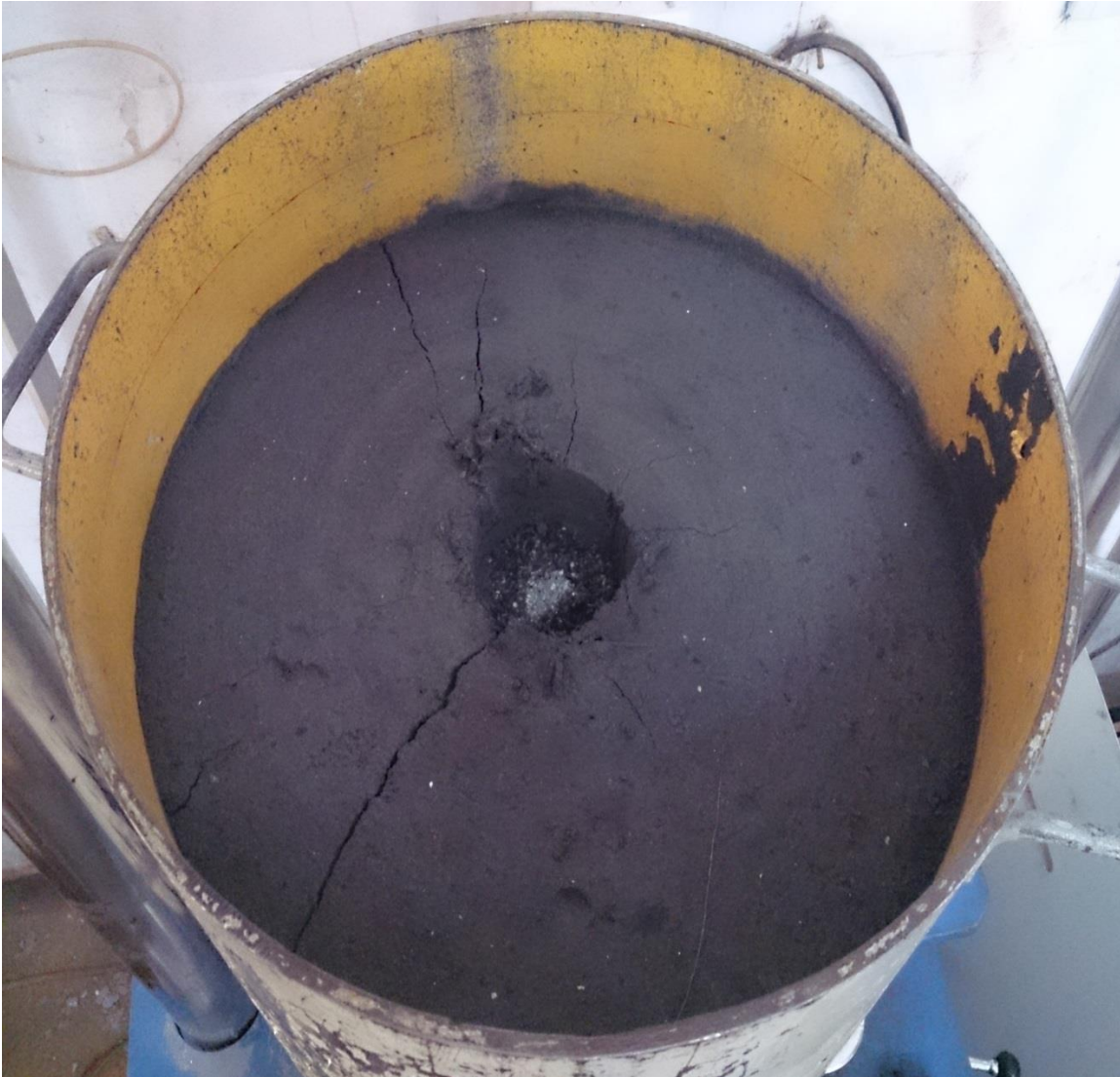
Fig 3.3 Failed pond ash sample
