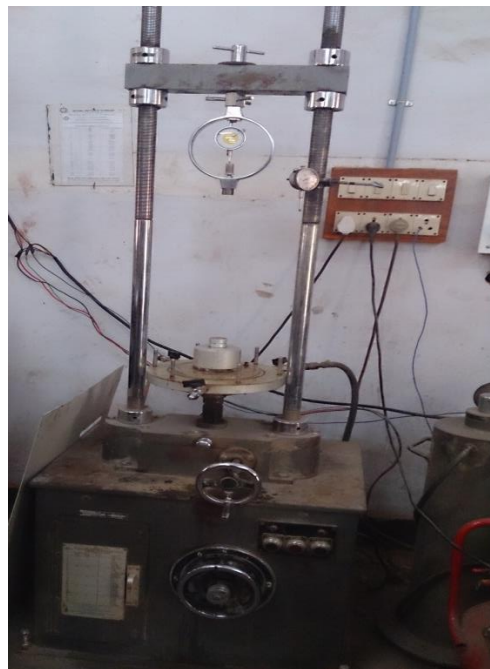
Fig 3.2 Footing Load test machine
