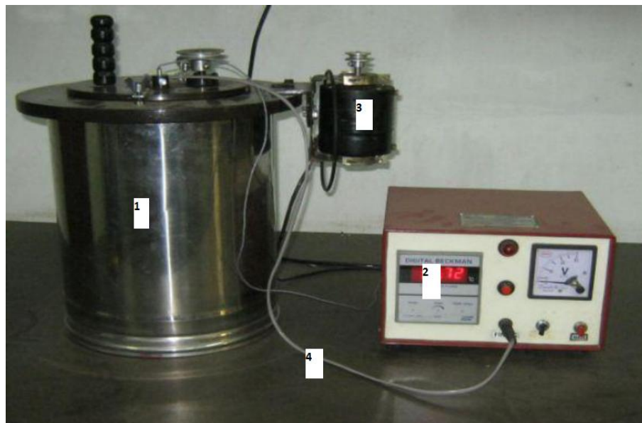
Figure 4.4 Photographic view of the bomb calorimeter apparatus
