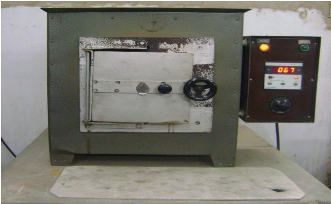
Figure 4.2: Photographic view of muffle furnace for Volatile matter and Ash content determination
