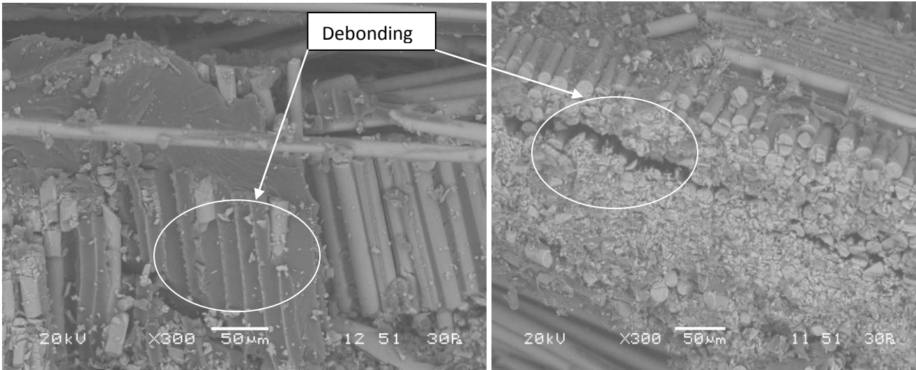
Fig. 4.12 SEM representing debonding
