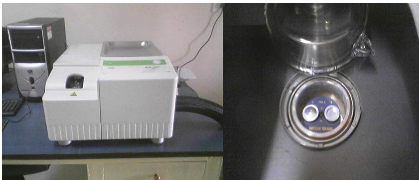
Fig. 2.8. Mettler -Toledo 821 with intra cooler for DSC measurements and reference sample chamber
