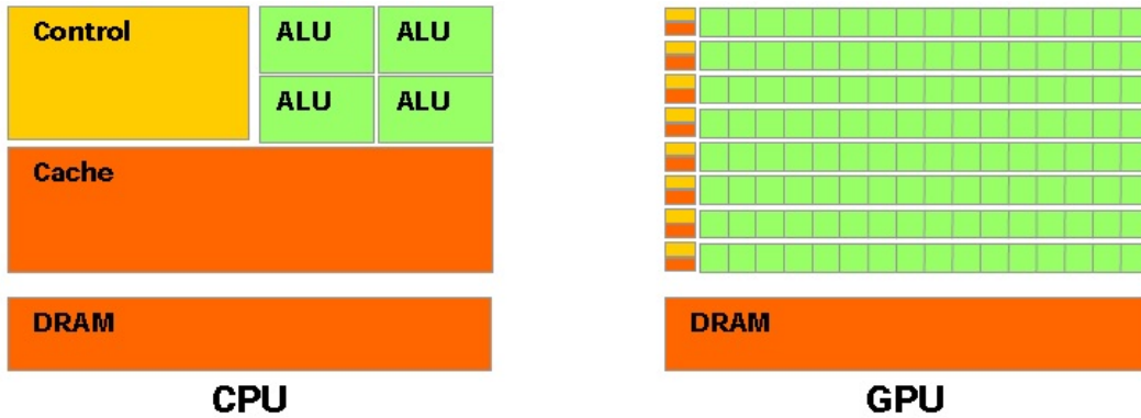
Figure 3.1: The GPU Devotes More Transistors to Data Processing
