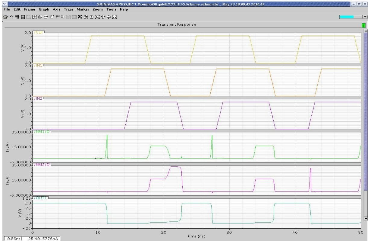
Fig. 4.4 Wide fan-in Domino OR gate-Footless schematic-Leakage current simulation.
