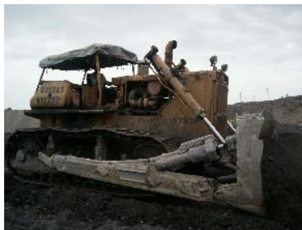
(e) Dozer (410hp)
