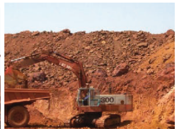
(f) Shovel ( 3m^3 bucket capacity, 320 hp)
