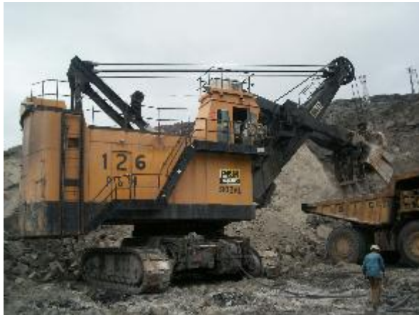
(c) Shovel ( 10\text{ m}^3 bucket capacity)
