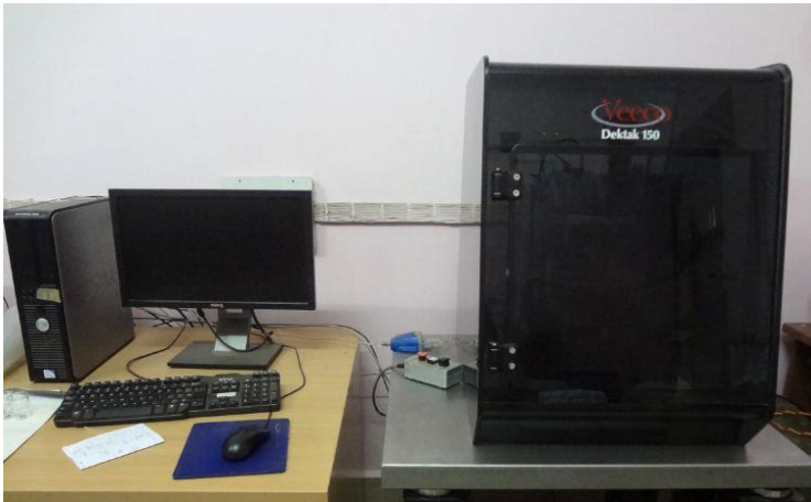
Figure 3.5: Stylus Profilometer Veeco Dektak, Electrometallurgy Lab, NIT Rourkela
