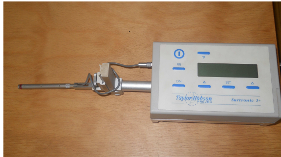
Fig. A.3: Talysurf Surface Roughness Analyser Brand : Taylor Hobson, Model : Surtronic 3 +
