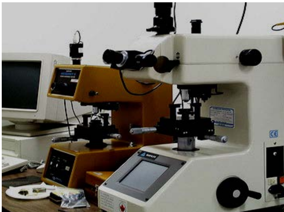
Fig. 4.10 Leitz micro-hardness tester
