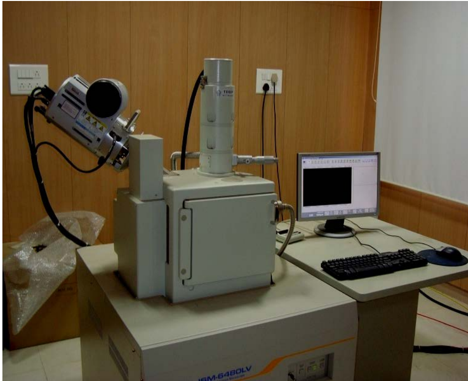
Fig. 4.9 Scanning Electron Microscope (JEOL JSM-6480LV)
