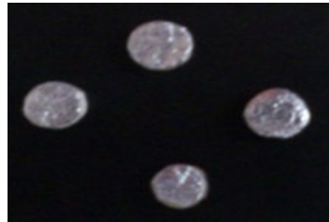
Fig. 4.19 Aluminium foil wrapped test samples for dielectric test
