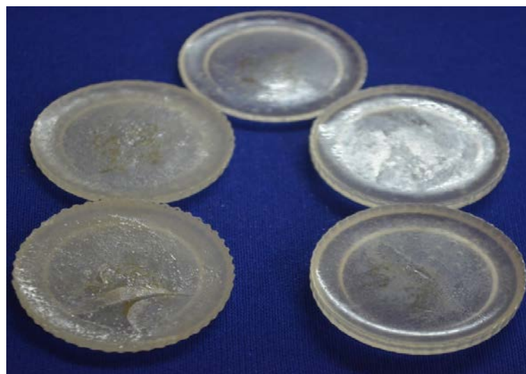
Fig. 4.7 Solid glass micro-spheres filled epoxy composites
