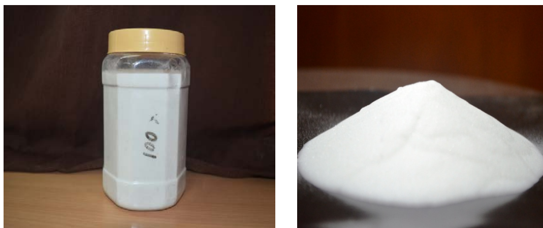
Fig. 4.4 Solid glass microspheres used as filler in the present work
