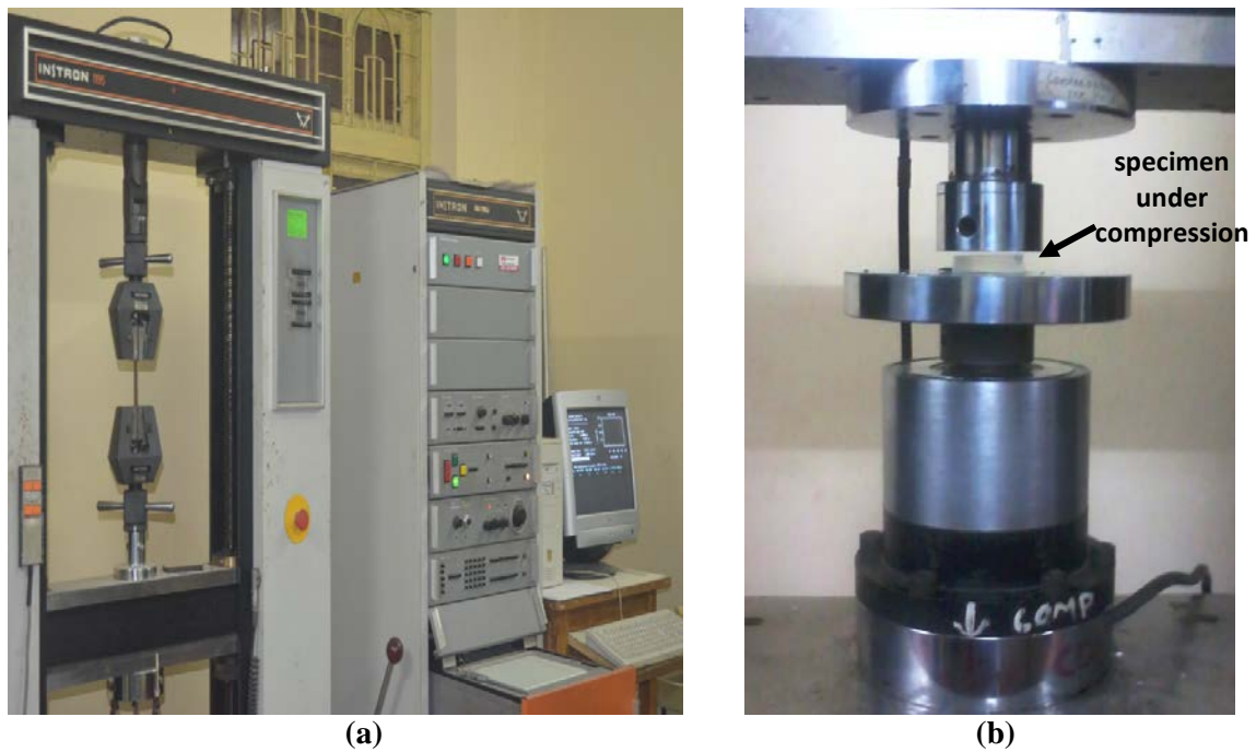
Fig. 4.12 (a) Universal testing machine Instron 1195 and (b) Loading arrangement for compression test
