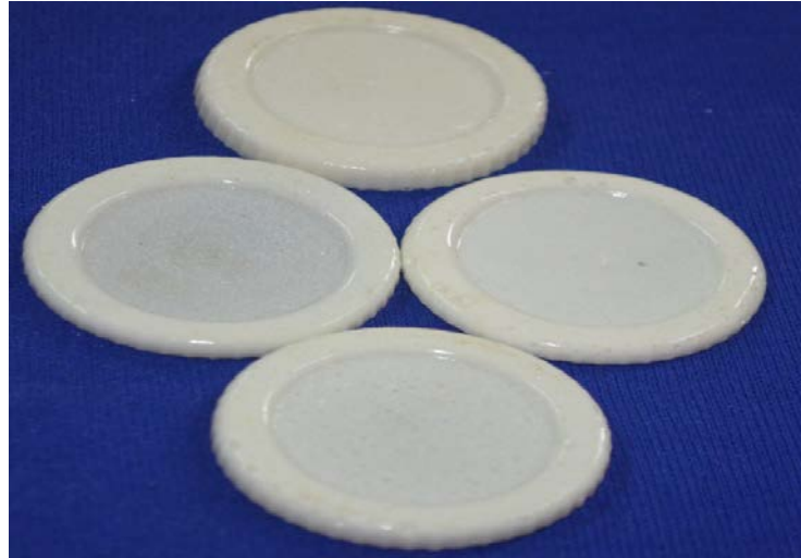
Fig. 4.8 Boron Nitride filled epoxy composites
