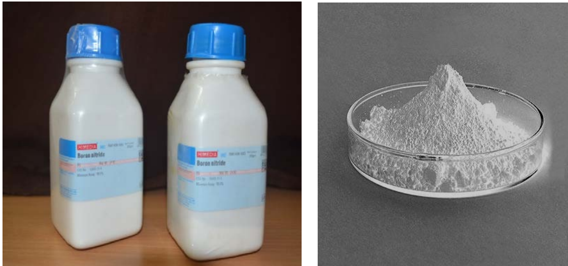
Fig. 4.5 Micro-sized boron nitride (BN) particles used as filler in epoxy
