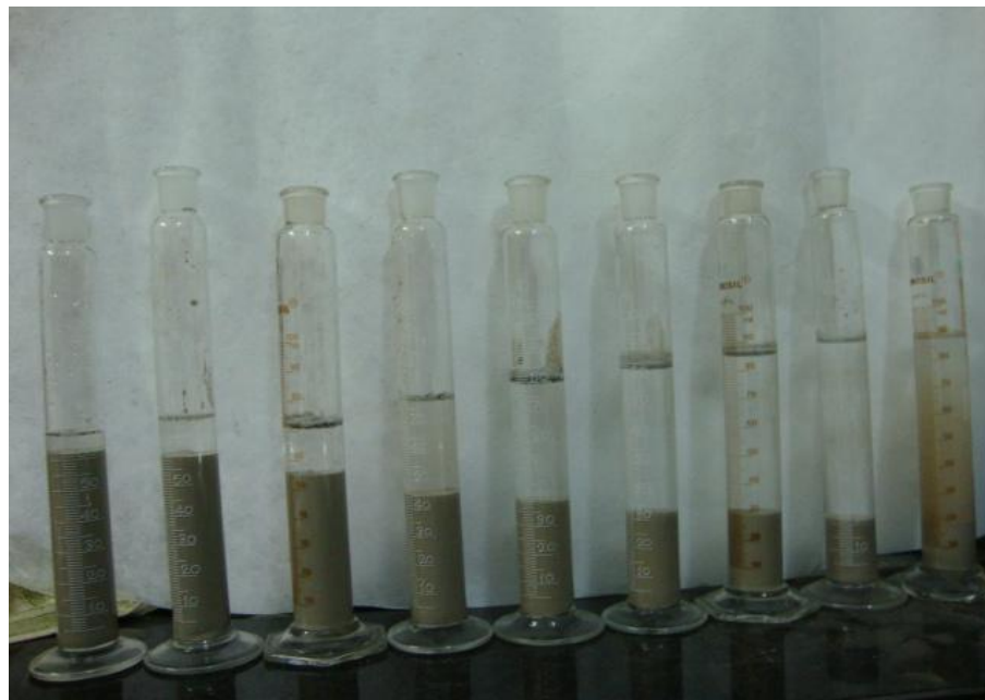
Figure 4.105: Settling study cylinders at varying doses of additives
