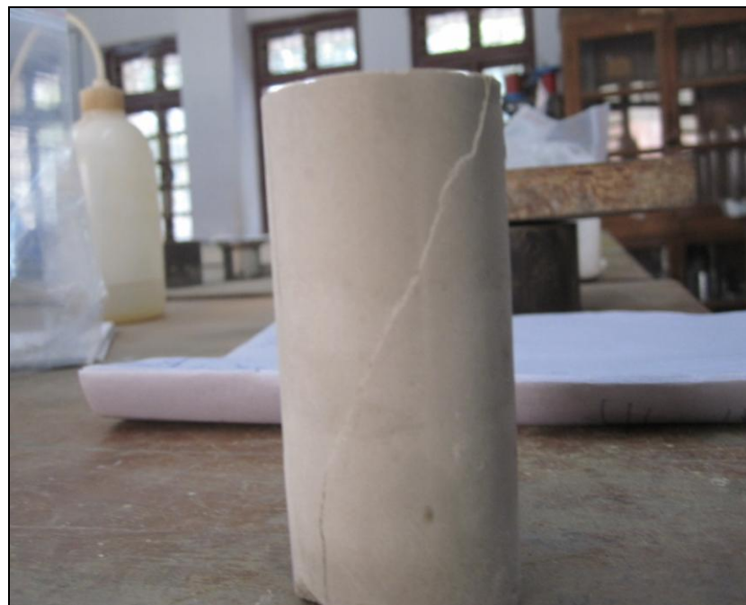
Figure 4.114: Post failure profile of a triaxial test specimen
