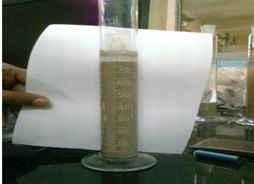
Figure 4.104: Settling study cylinder set up
