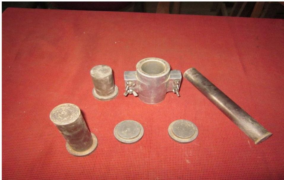
Figure 3.11: UCS mould for sample preparation
