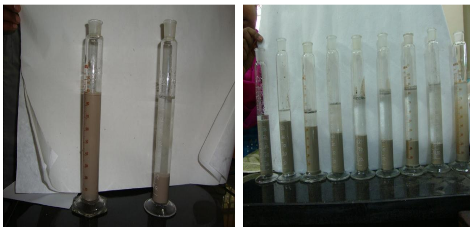
Figure 3.7: Settling study of fly ash slurry
