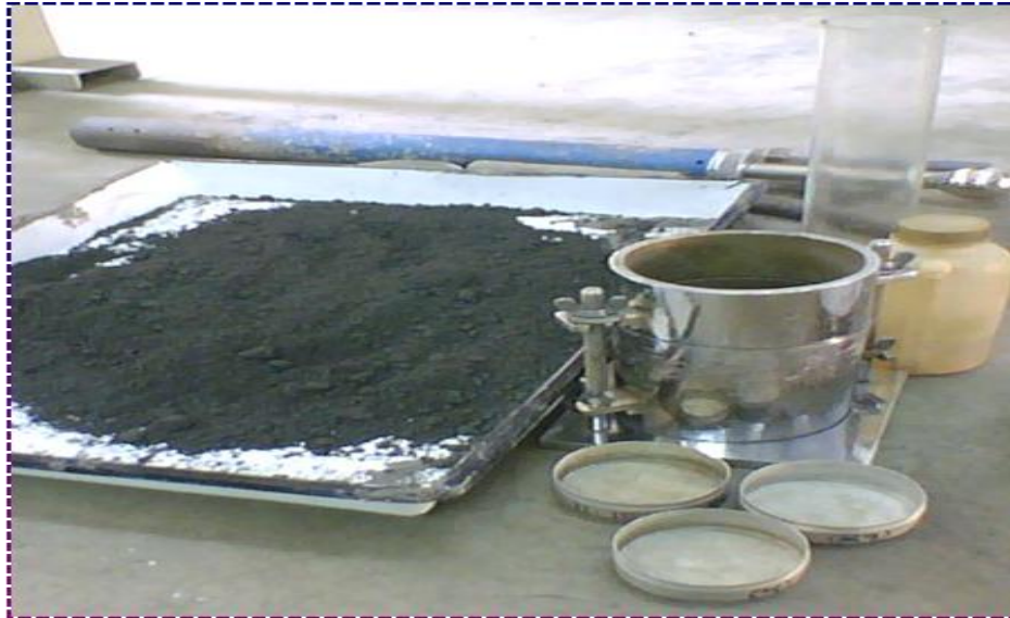
Figure 3.15: Sample preparation for proctor compaction test
