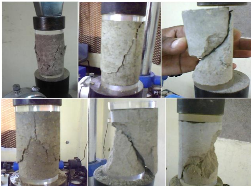
Figure 4.110: Post failure profiles of UCS samples
