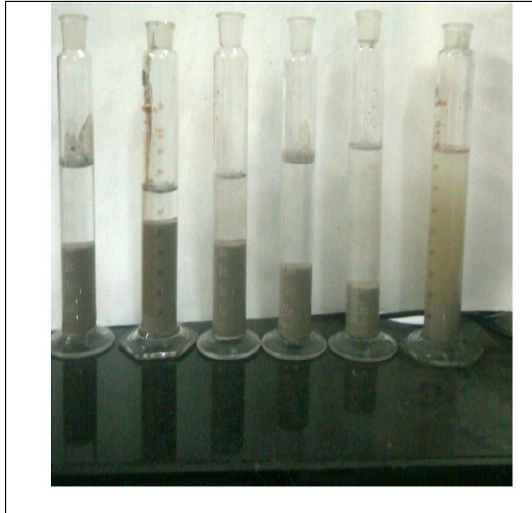
Figure 4.30: Settling results of fly ash slurry
