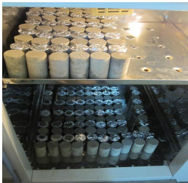
Figure 3.13: Sample of UCS specimens prepared (undergoing curing)
