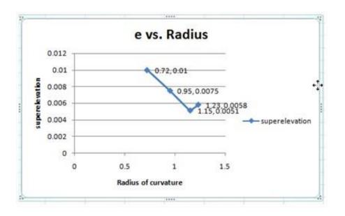
Max and Min values of superelevation(e)
