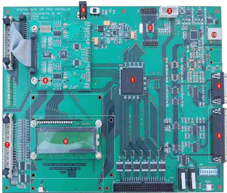
Figure 3.22: Spartan-3A DSP Trainer Kit with following components such as (1) SPARTAN-3A DSP Processor, (2) PLL Clock Setting, (3) JTAG Connector, (4) RS232 Serial Port, (5) Parallel Port, (6) LCD Display, (7) PWM Connector, (8) SDA Bus Connector, (9) Power Supply and (10) USB
