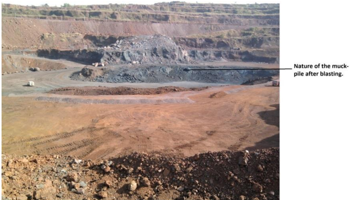
Figure No. 19 mine bench face after blasting operation
