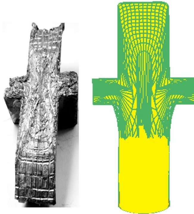
Figure 5.19 Flow pattern for forward-backward extrusion-forging process
