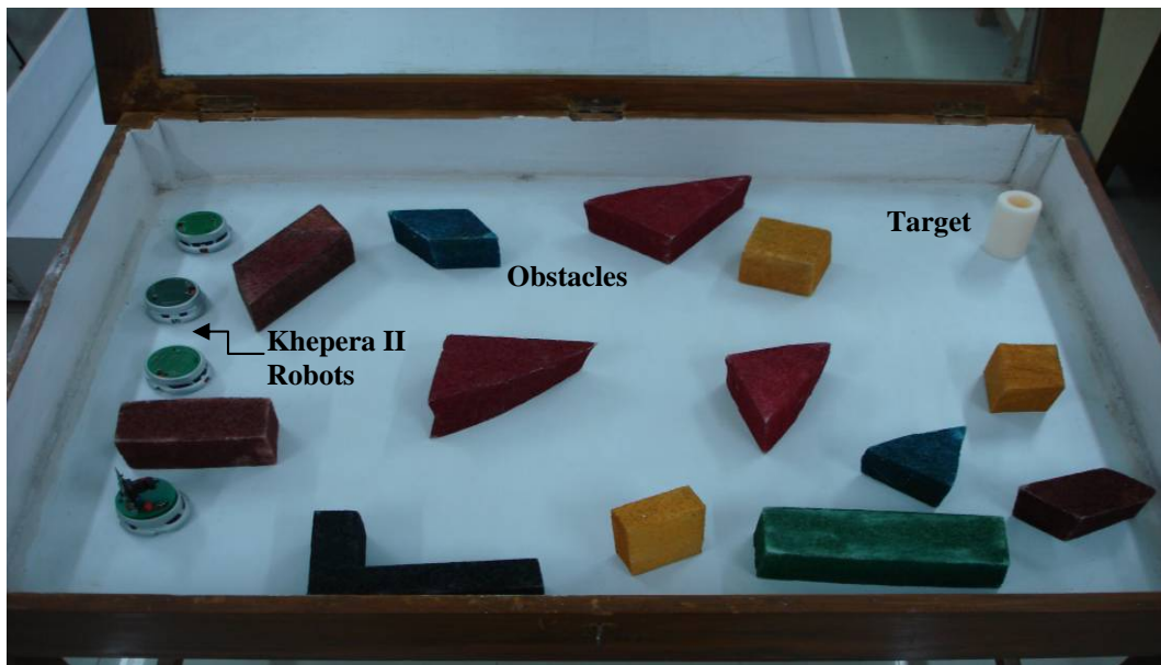
Fig. 6.36. Navigation of four real robots (Khepera II) in a cluttered environment (Initial scenario).
