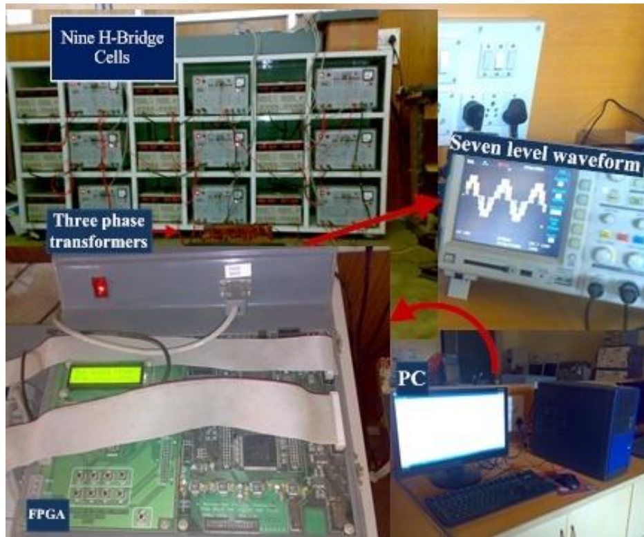
Fig.4.7 Details of Prototype set up for the proposed cascaded multilevel converter with three-phase transformers
