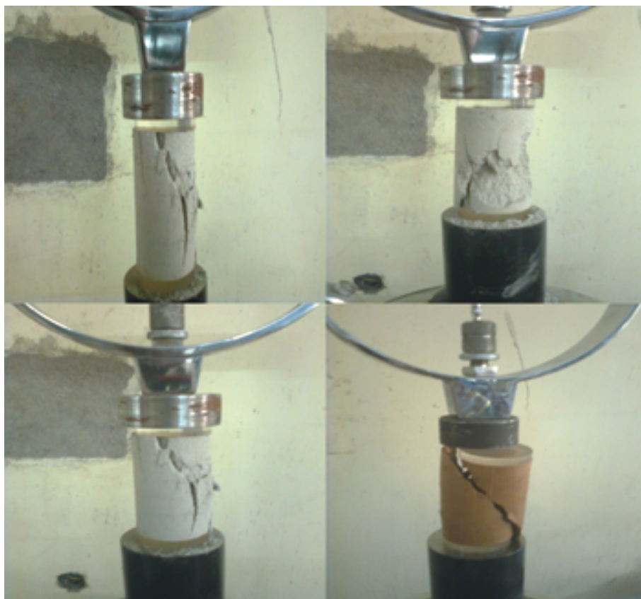
Figure 4.22: Post failure profiles of few UCS samples
