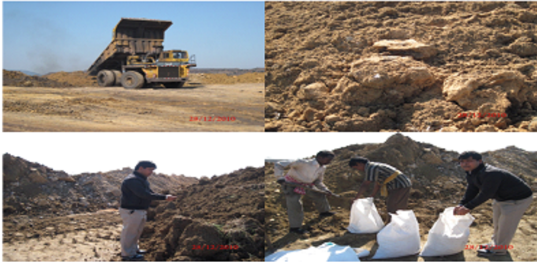
Figure 3.2: Collection of mine overburden samples
