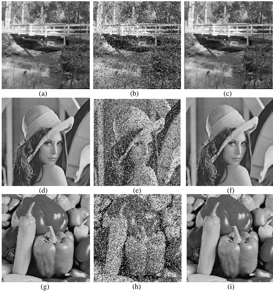
Fig.8.3. The original image (a)Bridge, (d)Lena, (g)Pepper and corresponding noisy image corrupted by 10%, 20%, 30% fixed value impulse noise is (b),(e),(h) respectively and (c),(f),(i) are filtered image of (b),(e),(h) respectively.
