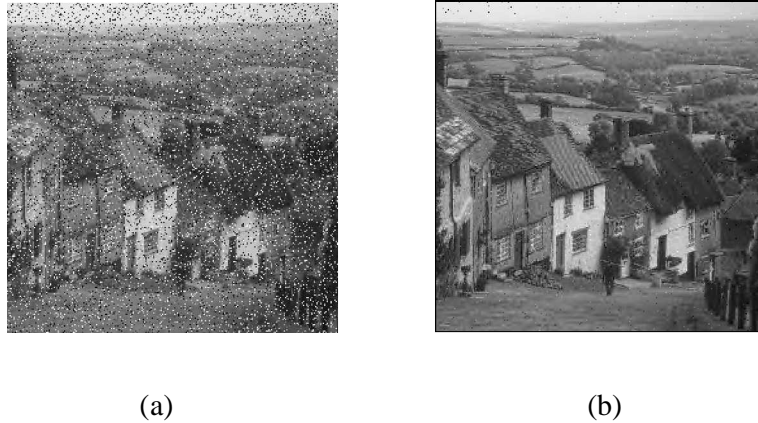
Fig. 5.2. Goldhill ( 512 \times 512) corrupted with random-valued impulse noise with 20% noise density in (a), and corresponding restored image in (b) .
