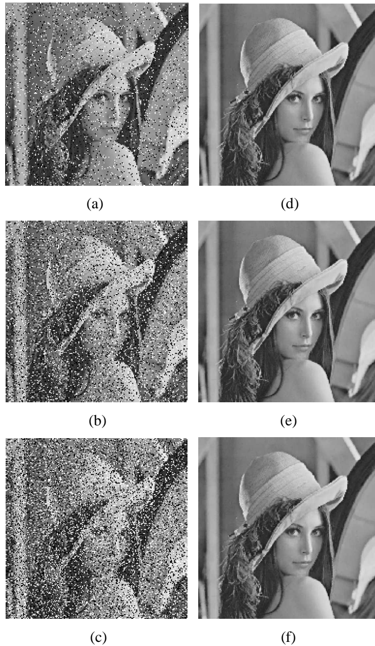
Fig. 5.3. Noisy images of Lena a, b, c with noise density of 10, 20, 30% and corresponding restored images d, e, f respectively
