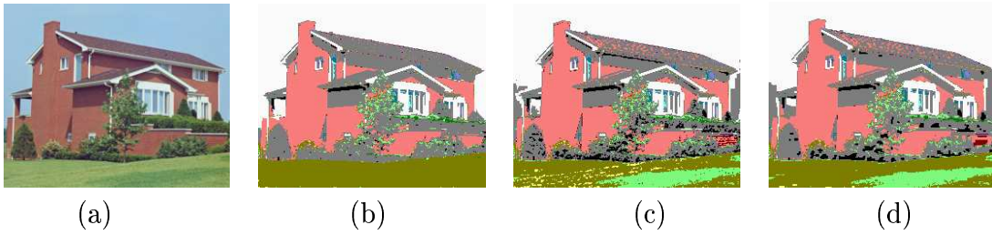
Figure 4.11: Segmentation of Scene image of size 256x256 using weak membrane model: (a) Original image (b) Ground Truth (c) MRF with Hybrid algorithm (d) DMRF with Hybrid algorithm
