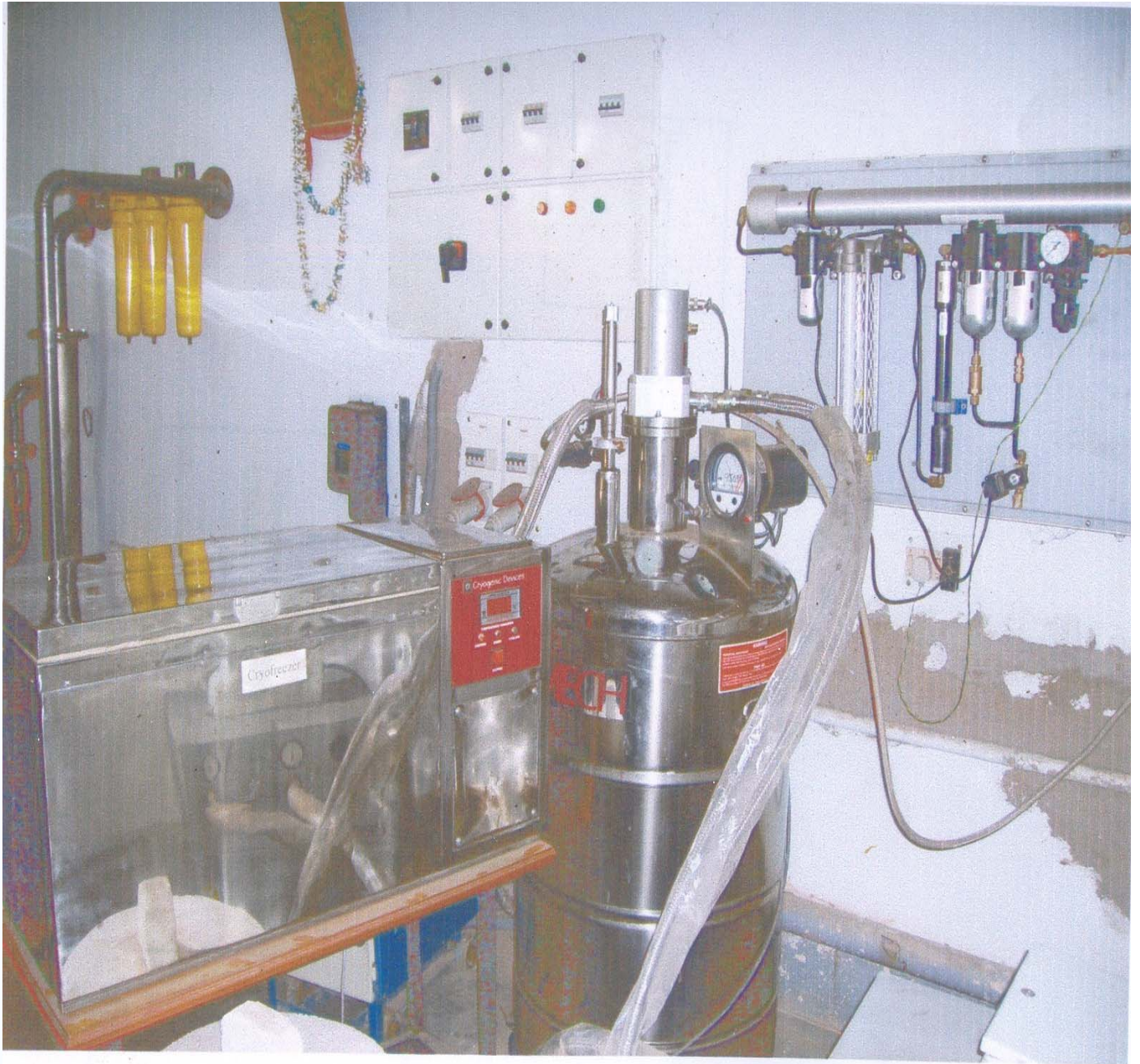
Fig. 3.5. Photograph of the cryogenic treatment set up
