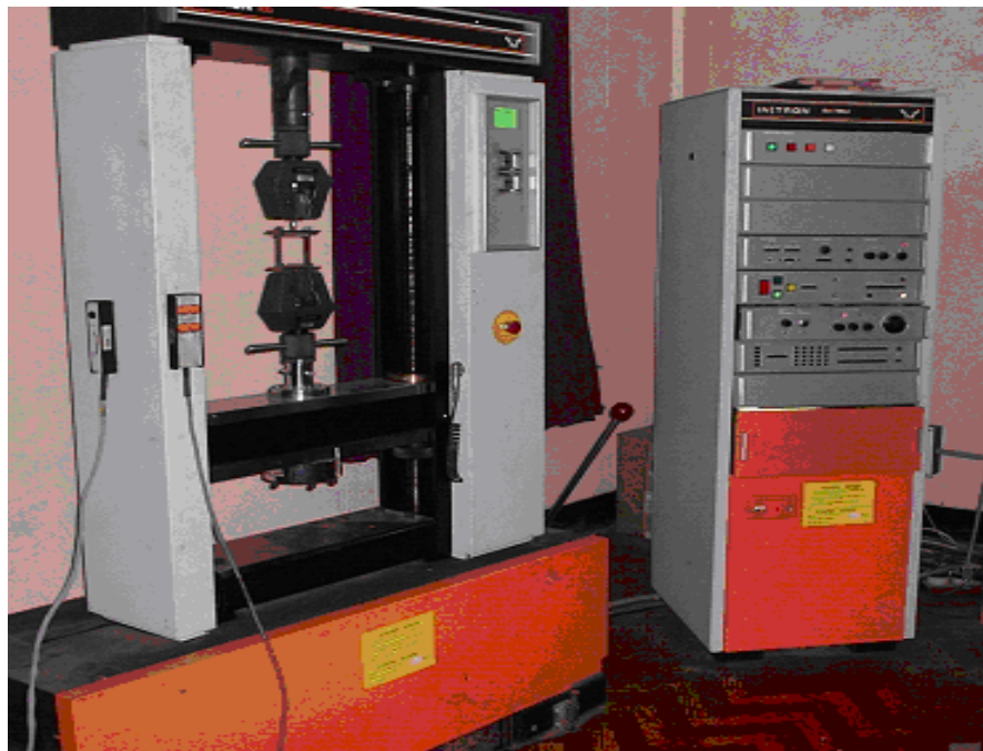
Fig 3.2 Testing machine with the specimen in loading position
