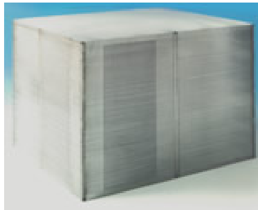
Figure1.3. Step 3. A block composed of diffusion bonded plates (courtesy HEATRIC™)
