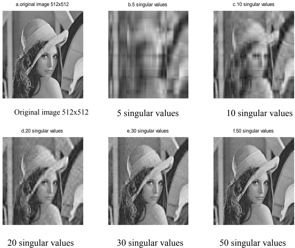
Figure 3.7. Approximation of images using SVD
