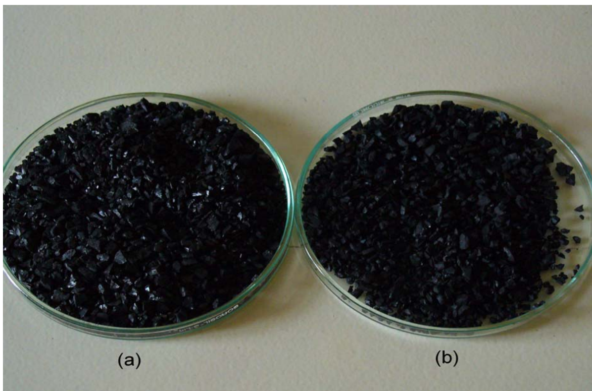
Fig 4.19: Activated Carbon catalyst Before (a) use and After (b) use
