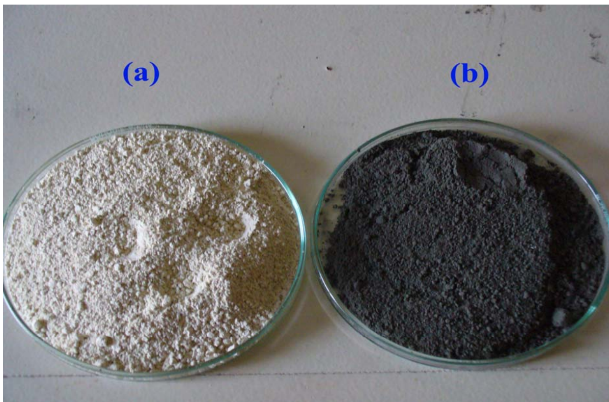
Fig 4.5: Silica Alumina catalyst before (a) use and after (b) use
