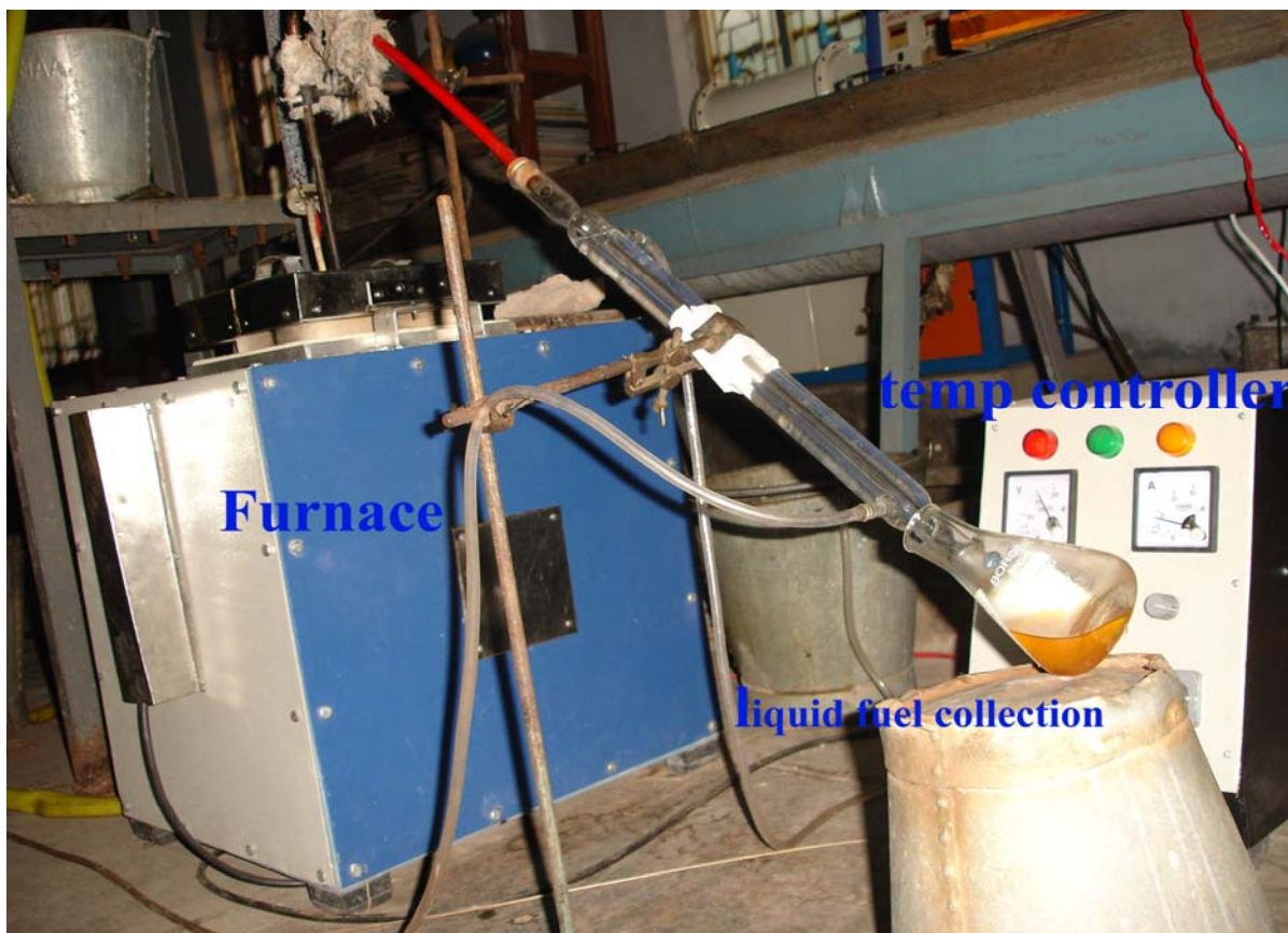
Fig 3.16: Experimental set up of Pyrolysis.
