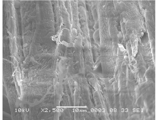
Fig. 4.17: SEM of 8h treated jute fibre composite at magnification 2500X.
