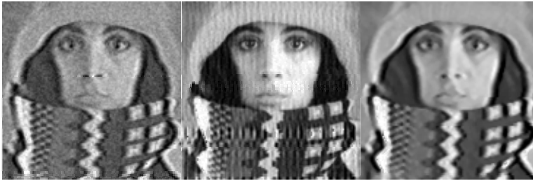
a) Distorted, noisy image b) Wiener filter c) Median filter ( 3 \times 3 )
