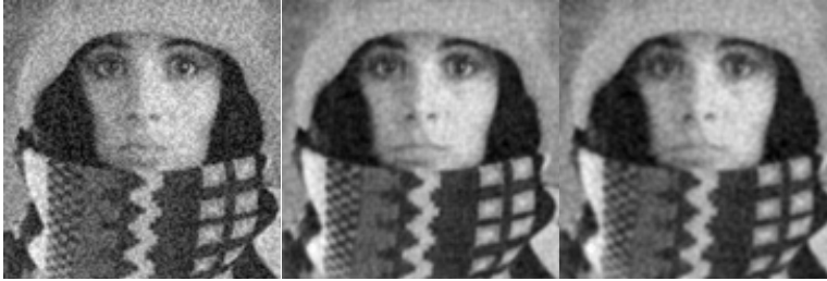
a) Noisy image ( SNR=20\text{ dB} ) b) Wiener filter c) Gauss filter ( \sigma = 1.0 )
