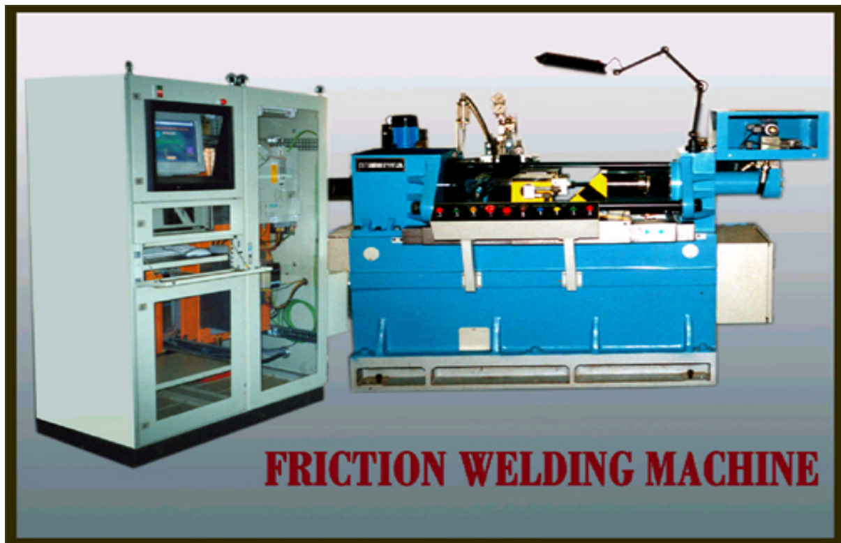
15 Ton Machine for welding axle housing of Trucks
