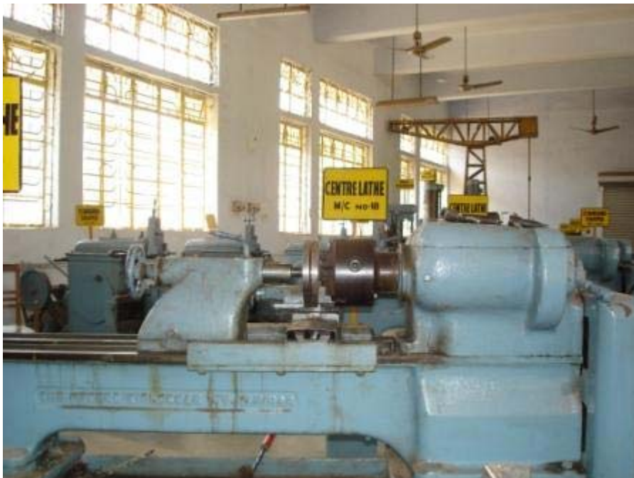
Fig-4 Experimental set-up for friction welding
