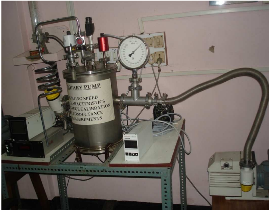
Fig 4.2 Apparatus Set in IIT KGP for measurement of pumping speed by constant volume method
