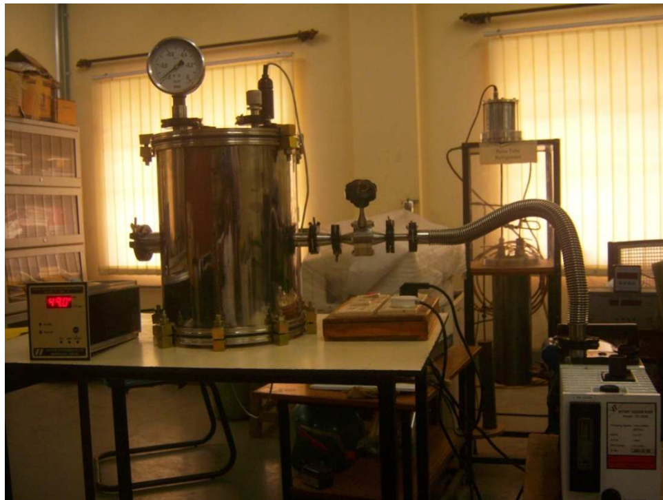
Fig 4.3 Apparatus Set in NIT RKL for measurement of pumping speed by constant volume method
