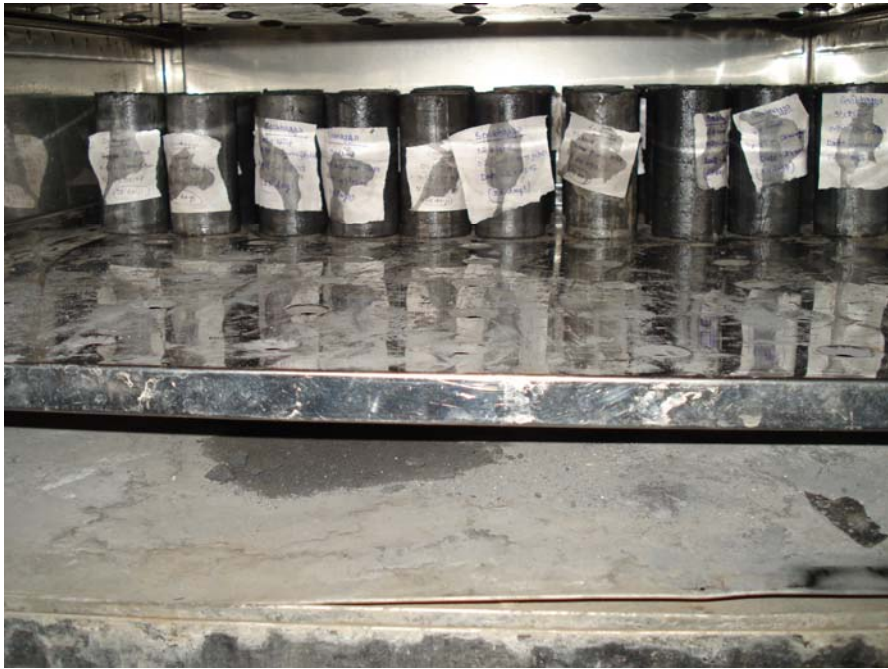
Samples inside humidity chamber
