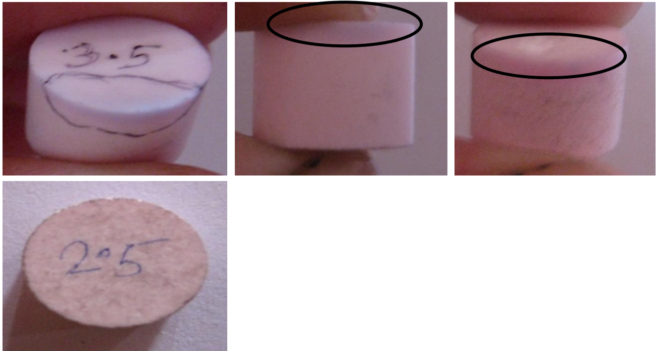
Fig. 4.2 Bluish colouration (left-most) and pink colouration of the pellets (two on right) . Dark spots persisting even after firing (bottom) . Regions showing impurity incorporation in pellets.
