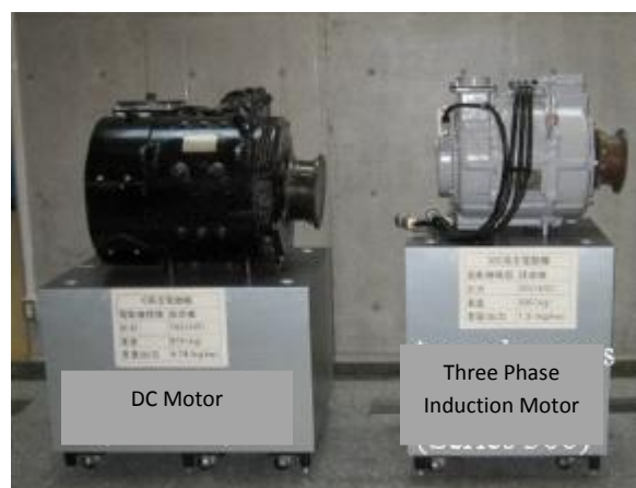
Fig 1.3 DC motor and Induction Motor
