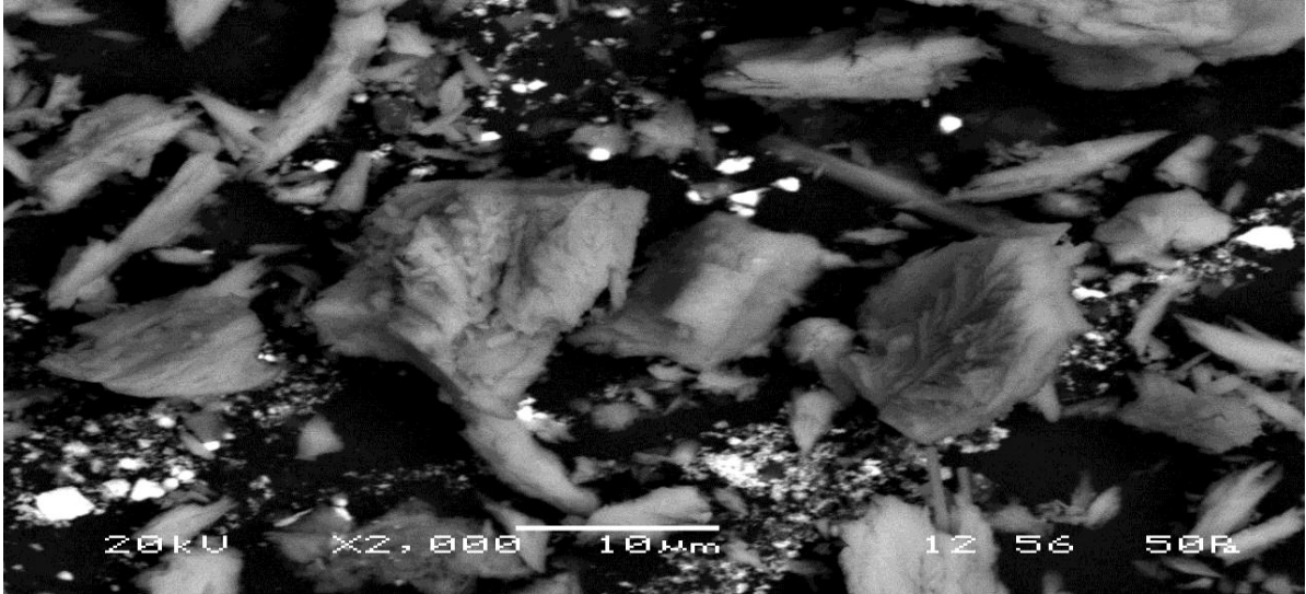
Fig. 5.8 Microstructure of plaster of Paris sample taken from the top part of the container.(X2000)shows that particles at top part of container are possessing angular structure with irregular surfaces.
