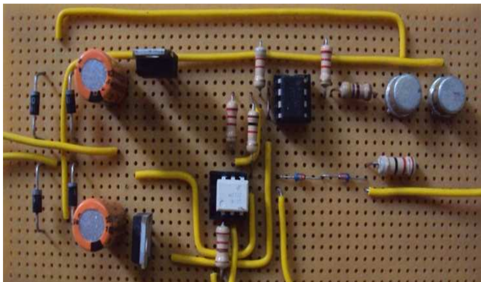
Figure 6.14 Gate drive circuit
