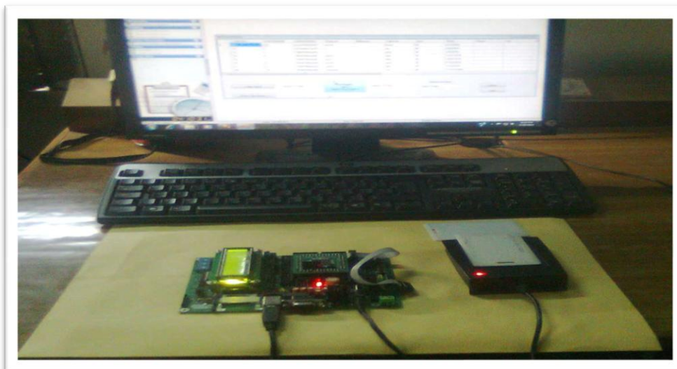
Figure 5.7 : Interfacing of RFID Reader, ATmega32 with PC.
