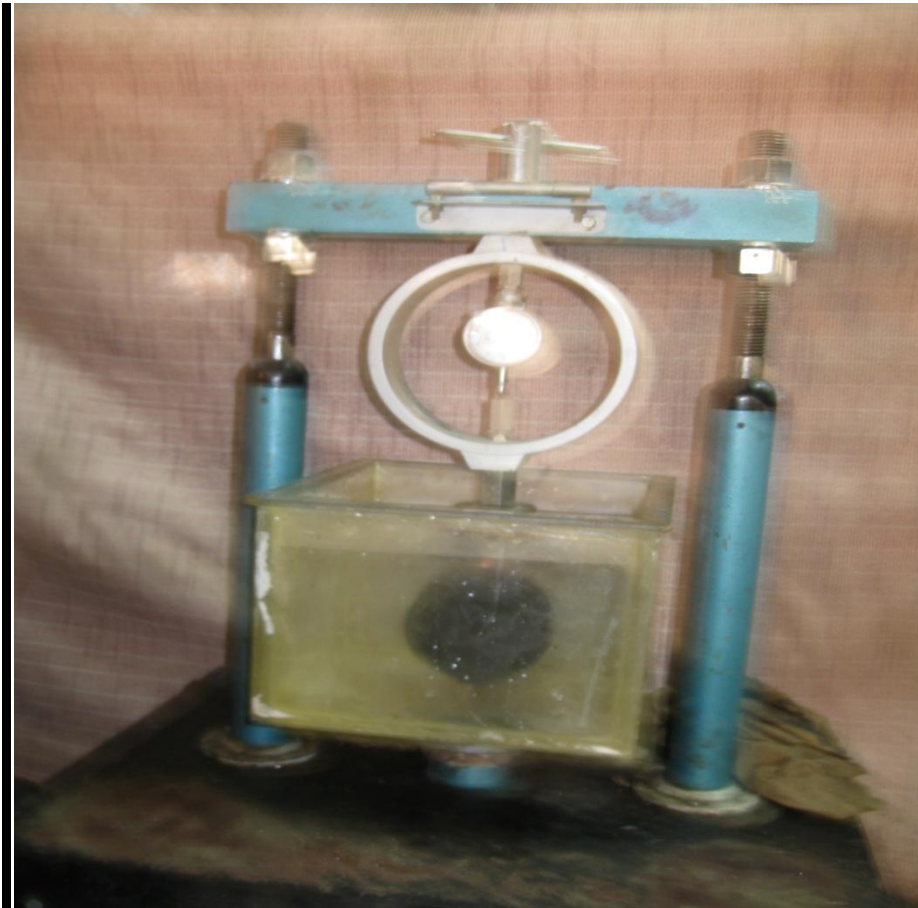
Fig 9. Static indirect tensile test
