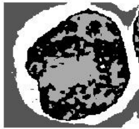
Figure 3.43: 4 clusters segmented image using k- means
