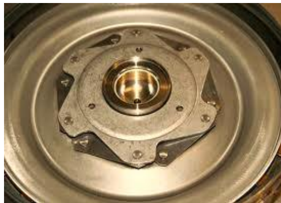
Fig 5 Friction welded piston clutch and impeller casting
