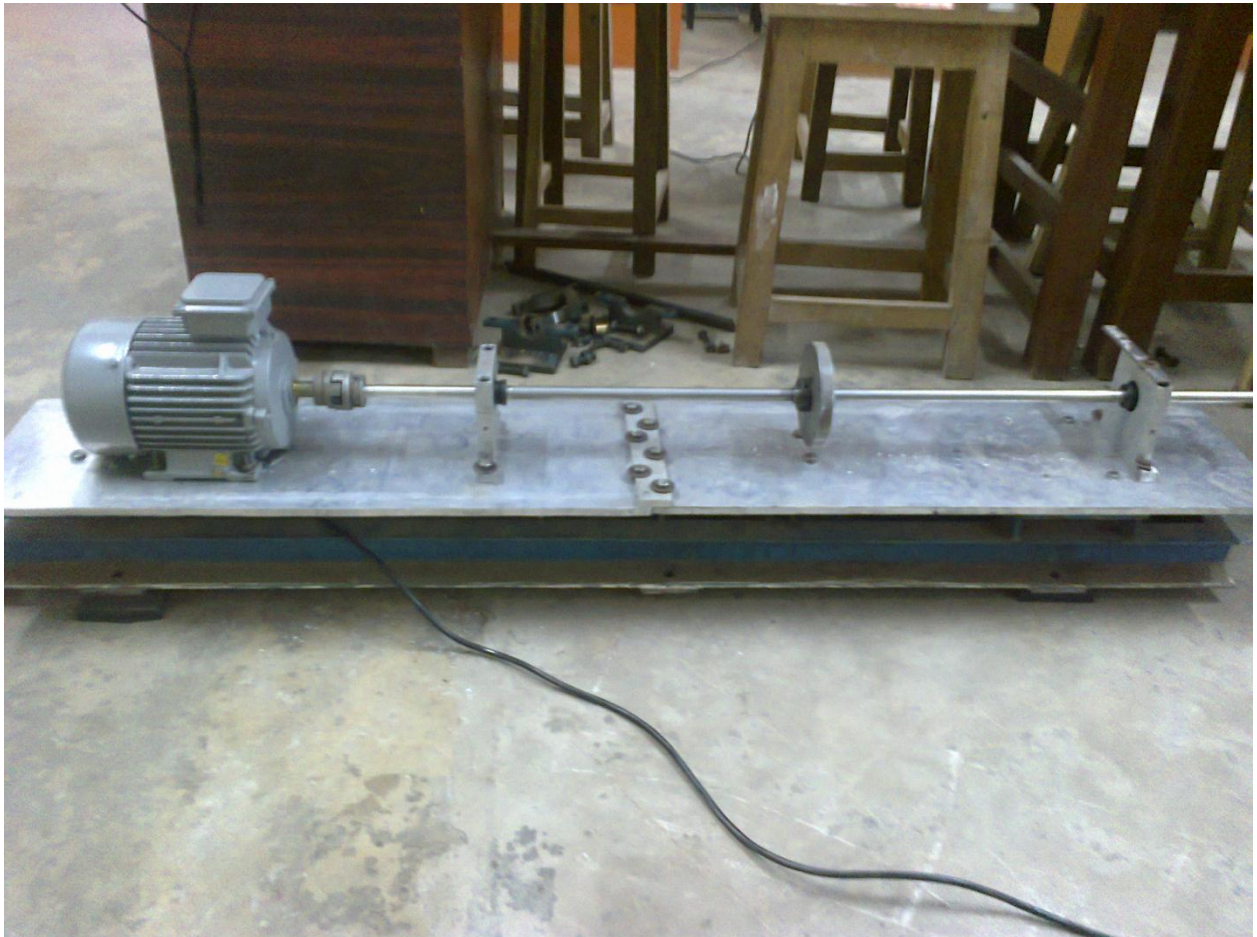
Fig 4.4 Solid Shaft held in between two Bearings
